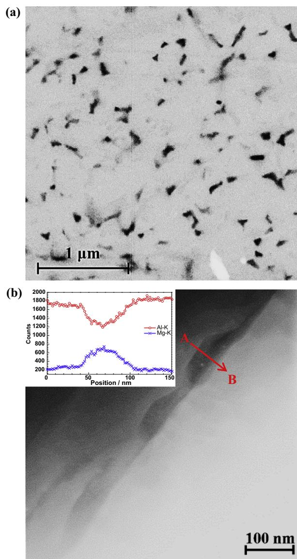
Fig. 1. (a) BSE micrograph showing morphology of A10 microelectrode after etching in 100 g/L  $(\text{NH}_4)_2\text{S}_2\text{O}_8$  for 2.5 h at room temperature; (b) typical HAADF (high angle annular dark field) micrograph of  $\beta$ -phase with Al and Mg concentration profiles across the line A–B.
