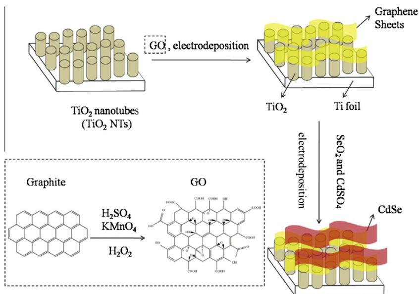
**Fig. 1.** Schematic diagram of procedures for preparing the CdSe/RGO/ $\text{TiO}_2$  composites.
