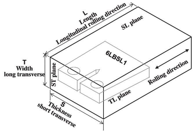
Fig. 1. Schematic of the orientation of 28% 1DCR 316NG SS and the alignment of CT specimen 6LBSL1.
