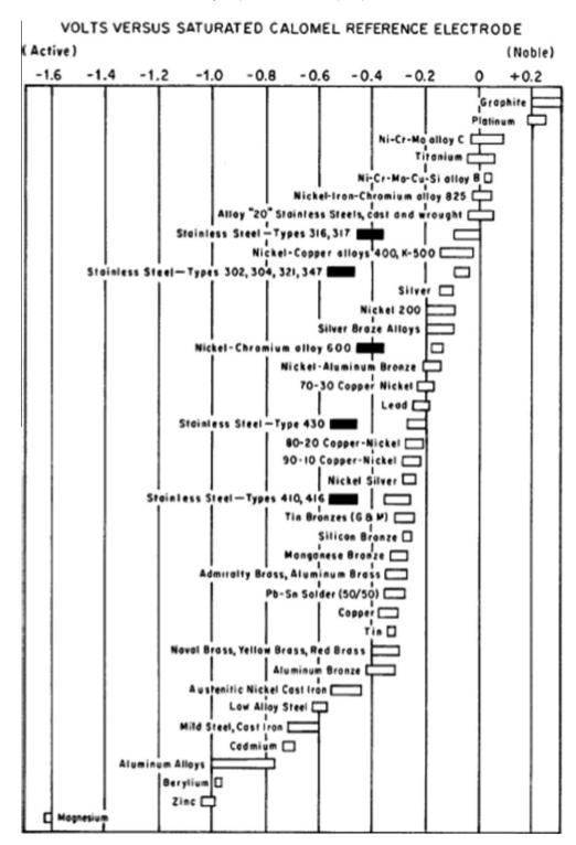
Fig. 1. Galvanic series where metals are ranked on the basis of the potential they exhibit in seawater at 2.4-4 m s<sup>-1</sup> for 5-15 days at 5-30 °C, as taken from ASTM G82 [1].
