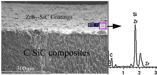
Fig. 2. EDS of  $ZrB_2$ -SiC coated C/SiC composites.
