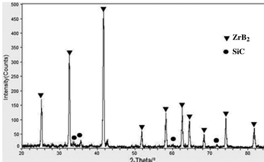
Fig. 3. XRD of  $ZrB_2$ -SiC coated C/SiC composites.
