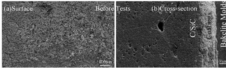
Fig. 1. SEM of  $ZrB_2$ -SiC coated C/SiC composites: (a) surface and (b) cross-section.
