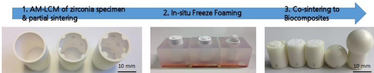
Fig. 1. Process scheme to co-manufacture Freeze Foam-filled LCM parts.
