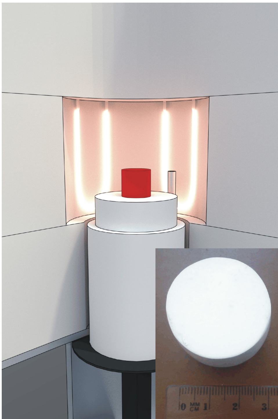
Fig. 1. Schematic of the furnace with the moving bottom table used for controlled insertion of the sample into the hot zone. Right down corner: the sample after rapid sintering.
