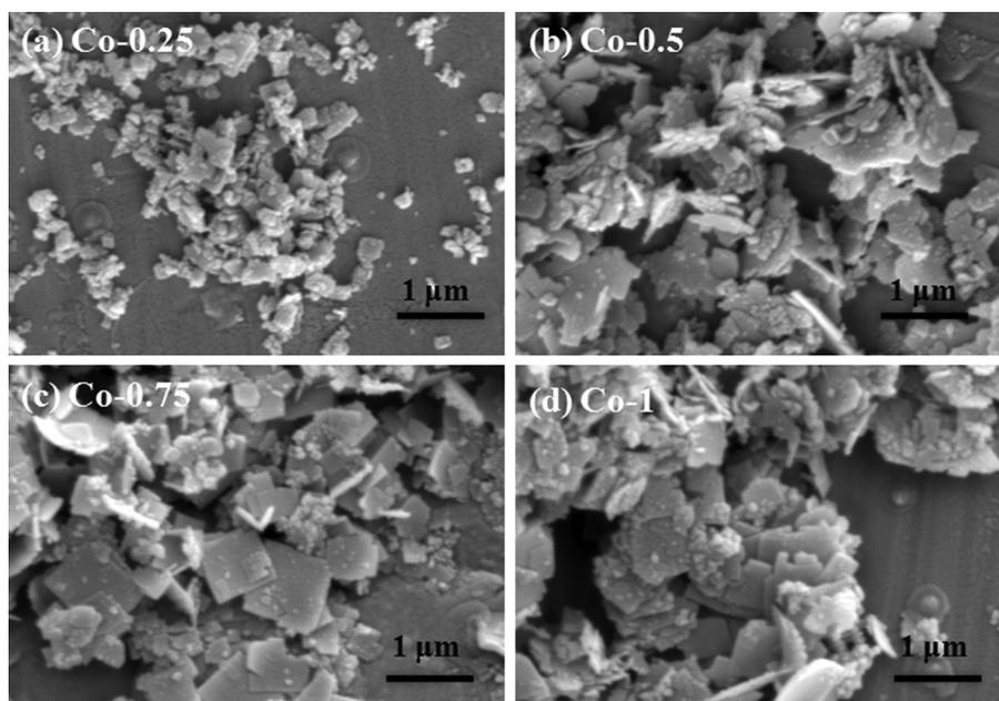
**Fig. 1.** SEM images of as-prepared BFCTO nanoplates with different cobalt content synthesized by hydrothermal method: (a) Co-0.25, (b) Co-0.5, (c) Co-0.75 and (d) Co-1, respectively.
