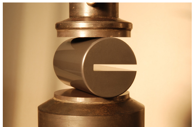
Fig. 2. Typical test setup in the Notched Roller Test. The roller is squeezed diametrically – the loading direction is perpendicular to the notch plane.
