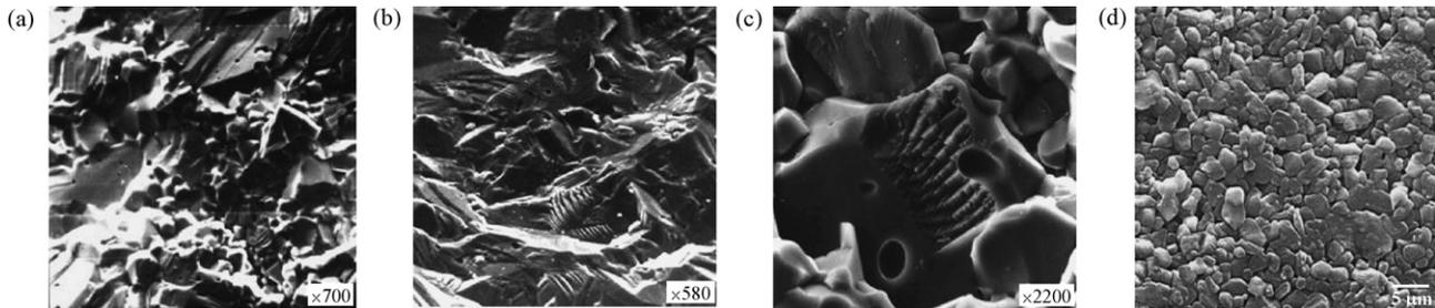
Fig. 1. Micrographs of fractured surfaces on S (a), Y (b), A-1 (c), and polished surface of A-2 (d) specimens.
