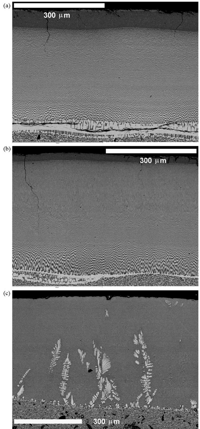
Fig. 1. SEM micrographs of polished transverse cross-sections of laser melt samples processed at increasing traverse speeds: (a) 20 mm/h; (b) 60 mm/h, and (c) 500 mm/h. Bright phase: YSZ; dark: NiO.
