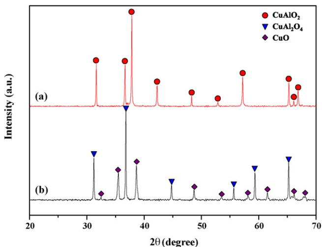
Fig. 1. X-ray diffraction patterns of the  $\text{CuAlO}_2$  disk target which was (a) quenched after sintering and (b) furnace cooled after sintering at 1200 °C for 4 h in air.
