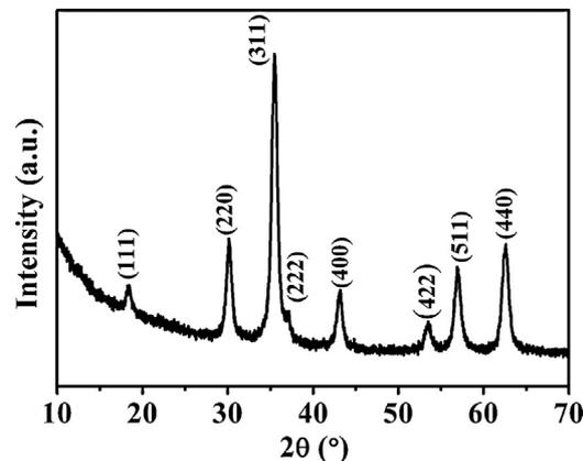
Fig. 1. X-ray diffraction pattern of 2 wt% CNT/Ni<sub>0.5</sub>Zn<sub>0.5</sub>Fe<sub>2</sub>O<sub>4</sub> composites hydrothermally treated at 200 °C for 3 h.
