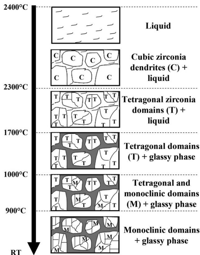
Fig. 1. Schematic representation of the microstructure of zirconia high containing refractory materials.
