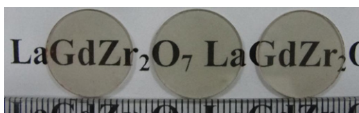
Fig. 2. Photos of LaGdZr 2 O 7 ceramics vacuum sintered at 1850 °C for 6 h and annealed at 1500 °C for 5 h in air (1 mm thick).
