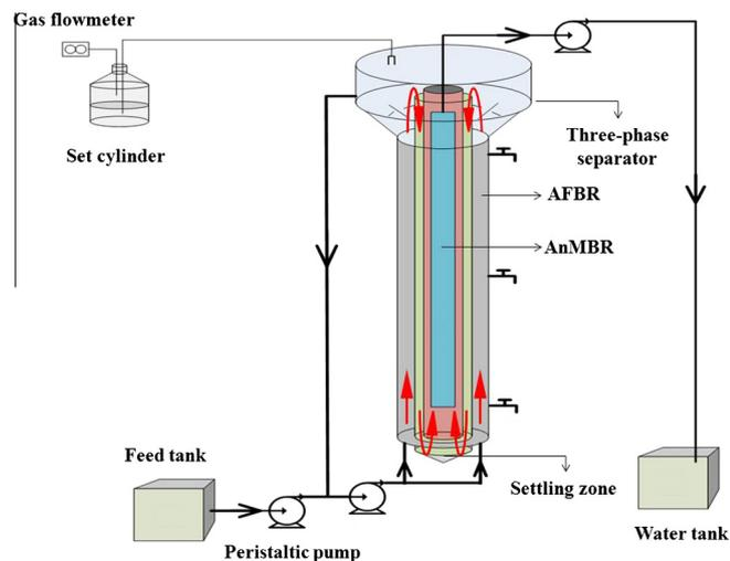
Fig. 1. Schematic diagram of integrated anaerobic fluidized bed membrane bioreactor (IAFMBR).
