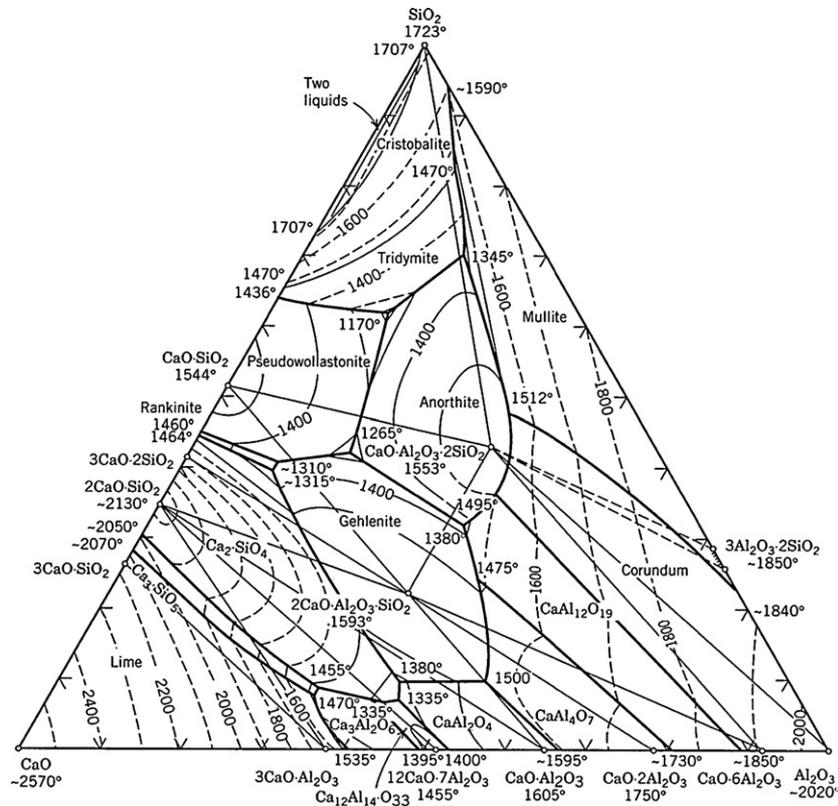
Fig. 1. CaO–Al<sub>2</sub>O<sub>3</sub>–SiO<sub>2</sub> phase diagram.<sup>1</sup>
