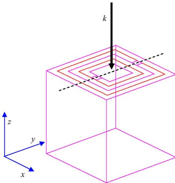
Fig. 1. Double slit tetragonal resonators with unit cell size  $1.2 \text{ mm} \times 1.2 \text{ mm} \times 1.2 \text{ mm}$ . The size of the tetragonal resonators is  $1.0 \text{ mm} \times 1.0 \text{ mm}$  for the outer and  $0.6 \text{ mm} \times 0.6 \text{ mm}$  for the inner one. The size of both tetragonal slits is  $0.1 \text{ mm} \times 0.1 \text{ mm}$ . Axis of slits is shown.
