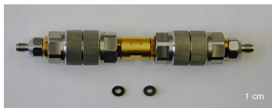
Fig. 2. Test fixture for transmission–reflection measurements of cylindrical hexaferrites.
