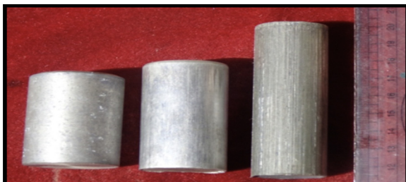
Fig. 1 – Photograph of specimens with different levels of extrusion (left to right: \epsilon = 0 , \epsilon = 0.266 , \epsilon = 0.305 ).
