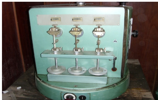
Fig. 1 – Device for testing on fatigue.
