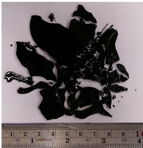
Fig. 1. The macrograph of 20B 2 O 3 -10SiO 2 -45BaO-25Fe 2 O 3 sample after quenching between two cold steel sheets.
