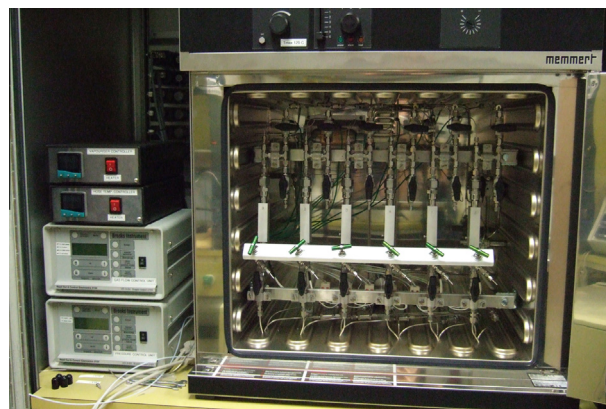
Fig. 2. Picture of parallel reactor system used to study the activities and selectivities of different ring opening catalysts.
