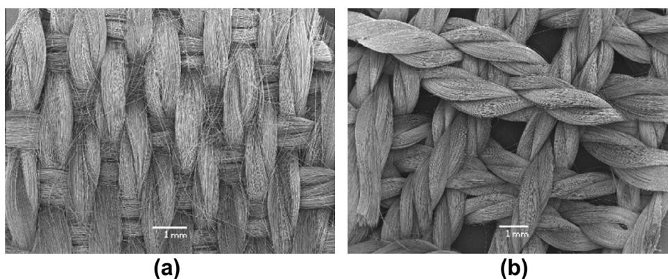
Fig. 2. Sample photo of fiber-glass fabrics: (a) sateen type and (b) "false openwork" (lightweight) type.
