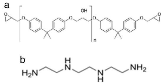
Fig. 1. (a) Structure of unmodified epoxy pre-polymer resin. (b) Structure of a hardener.
