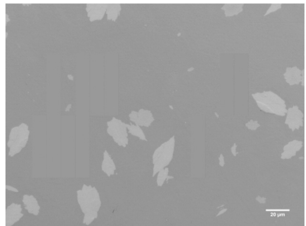
Fig. 2. Optical micrograph of a lithium disilicate glass-ceramic obtained by annealing glassy lithium disilicate for 90 h at 500 °C.
