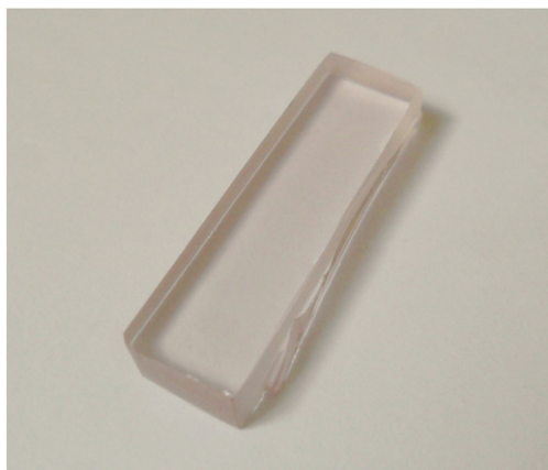
Fig. 1. Glass M1. The lower part is coated with sol–gel silica coating (sample size 8 × 30 mm 2 ).
