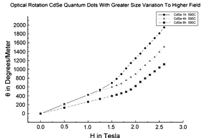
Fig. 1. Optical rotation of CdSe quantum dots with less homogeneity and greater size dispersion (~30%). (Estimated error from averaging a number of data runs is  $\pm 50$  °/T-Meter).
