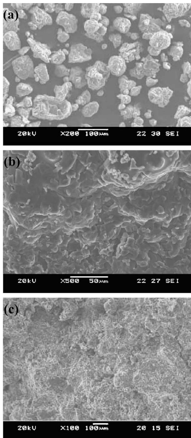
Fig. 1. SEM micrographs of (a) raw mixtures, (b) waterish mixtures, and (c) dense mixtures.
