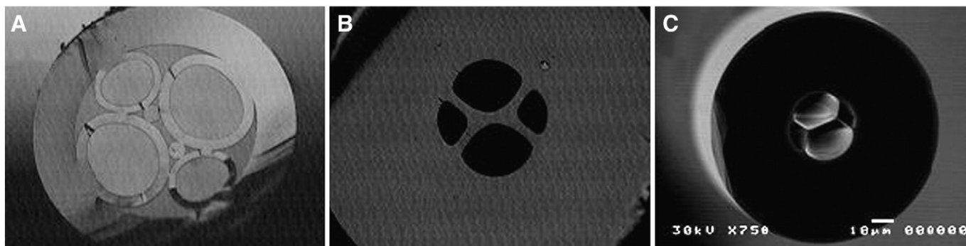
Fig. 1. Cross section images showing different stages of the MOF manufacturing process: (A) preform stage with four capillaries and two rods stacked inside a silica tube (before air evacuation of interfaces); (B) a cane with a structure similar to that of the desired MOF; and (C) final structure of the MOF, with \sim 110\ \mu\text{m} external and \sim 2.5\ \mu\text{m} core diameters.
