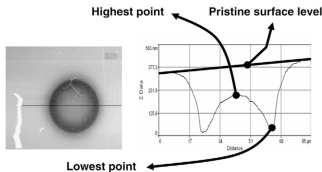
**Fig. 1.** A typical AFM picture of the irradiated glass surface spot (left). The line shows the track of the following scan, results of which are on right. The processing of scan is visualized (right); first the surface is levelled by the linear fitting of the unirradiated sides, then the lowest and highest points are determined.
