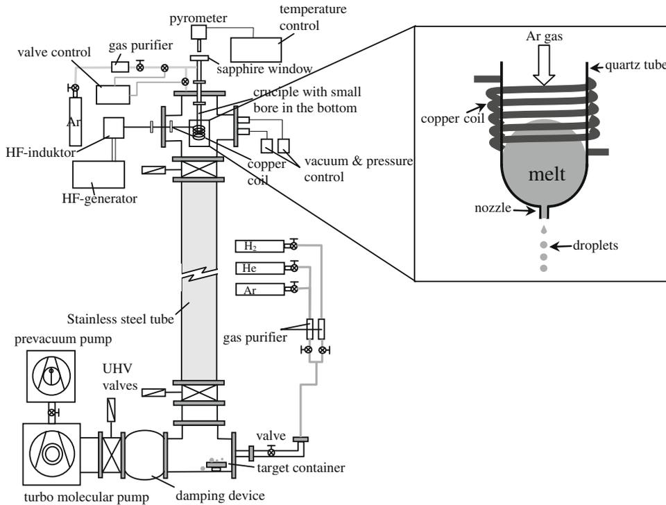
Fig. 1. Schematic illustration of the drop tube.
