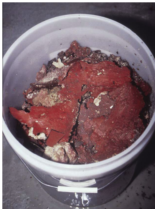
Fig. 1. Pieces of antifouling paint removed from the grounding site [22].
