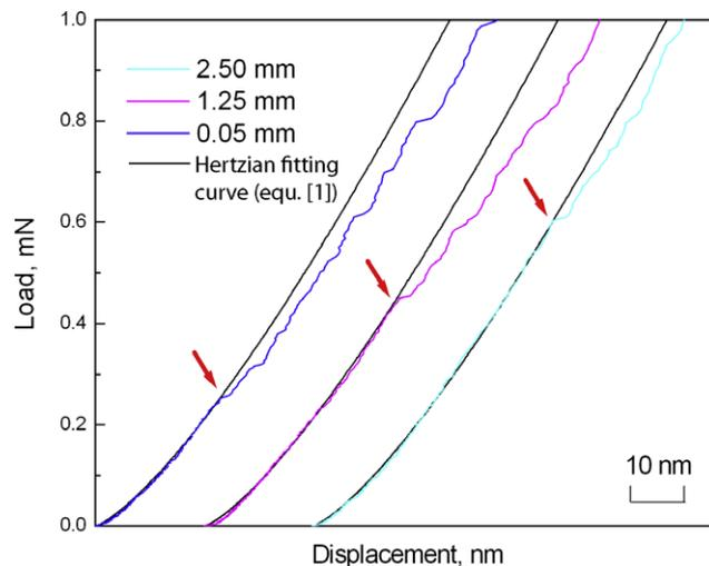
Fig. 4. Initial nanoindentation response of three indents located 0.05, 1.25, and 2.5 mm from the edge of the as-cast  $\text{Ti}_{40}\text{Zr}_{25}\text{Ni}_3\text{Cu}_{12}\text{Be}_{20}$  glassy sample for a depth of 500 nm. In each case, the first portion of the experimental data can be well described by the Hertzian elastic contact law (solid black lines), but the departure from ideal elasticity occurs earlier for samples at smaller loading rates or with smaller sizes.
