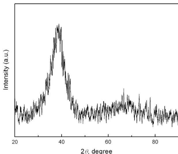
Fig. 1. XRD pattern for the as-cast  $\text{Ti}_{40}\text{Zr}_{25}\text{Ni}_3\text{Cu}_{12}\text{Be}_{20}$  bulk sample with a diameter of 5 mm.
