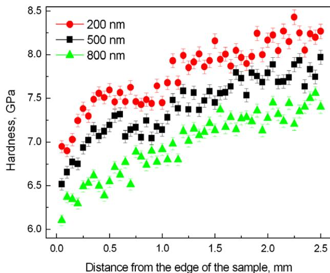
Fig. 2. Hardness of the as-cast  $\text{Ti}_{40}\text{Zr}_{25}\text{Ni}_3\text{Cu}_{12}\text{Be}_{20}$  bulk glassy alloy measured by nanoindentation.
