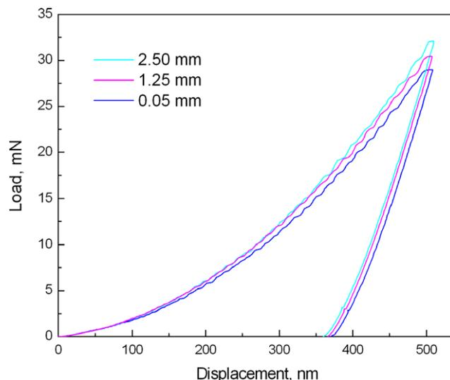
Fig. 3. Load–displacement curves of three indents located at 0.05, 1.25, and 2.5 mm from the edge of the as-cast  $\text{Ti}_{40}\text{Zr}_{25}\text{Ni}_3\text{Cu}_{12}\text{Be}_{20}$  glassy sample for a depth of 500 nm.
