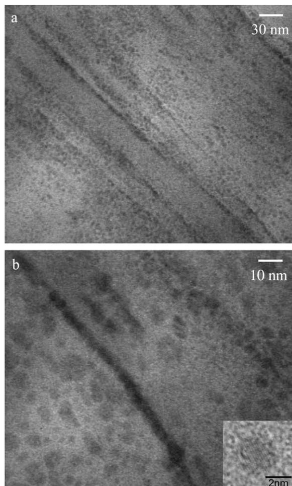
**Fig. 1.** (a) A typical TEM image showing the silver nanoparticles that, in some cases, assembled into elongated and well-aligned structures. (b) HREM image evidences isolated nanoparticles and nanoparticles aggregated into nano-ribbon, in the inset, the lattice image clearly evidences the crystalline nature of the nanoparticle.
