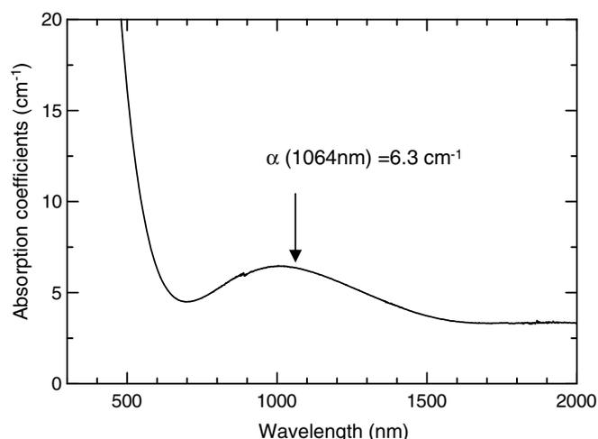
Fig. 2. Optical absorption spectra at room temperature for the 0.6FeO-BTG50 glass.
