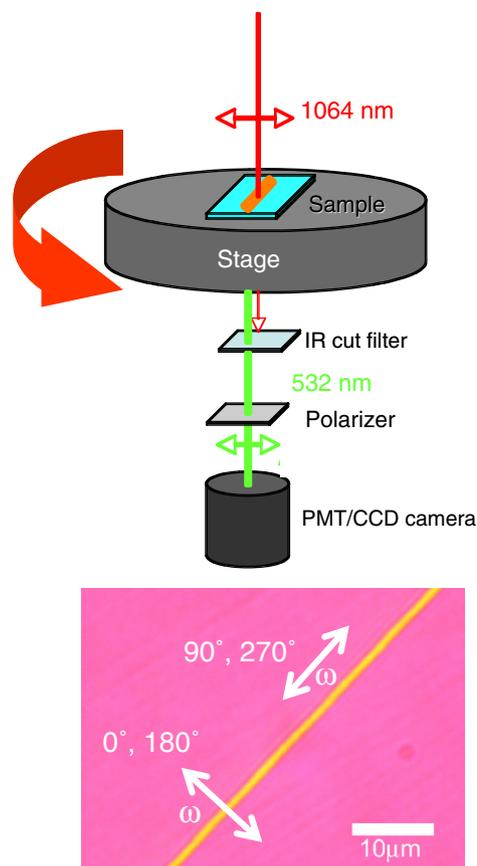
Fig. 1. Configurations of sample and incident laser for azimuthal dependences of SH intensity by second harmonic microscope. We decided the azimuth of  $0^\circ$  ( $180^\circ$ ) which polarization of fundamental wave ( $\omega$ ) is normal to the scanning direction.
