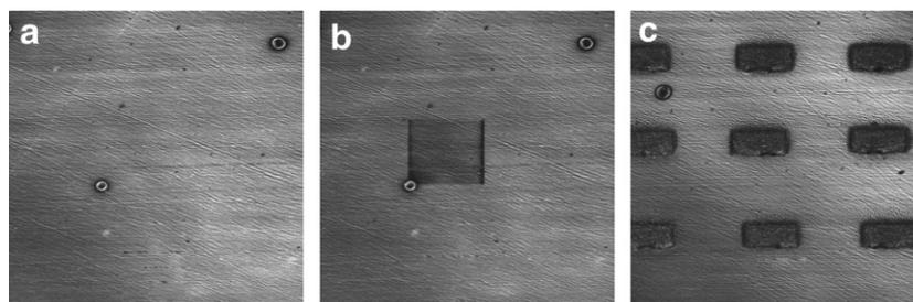
Fig. 1. Confocal images ( $274 \mu\text{m} \times 333 \mu\text{m}$ ) of (a) ‘as-deposited’  $\text{a-WO}_3$  thin film (b) after recording with 25 mW laser power and (c) after recording with 50 mW laser power.
