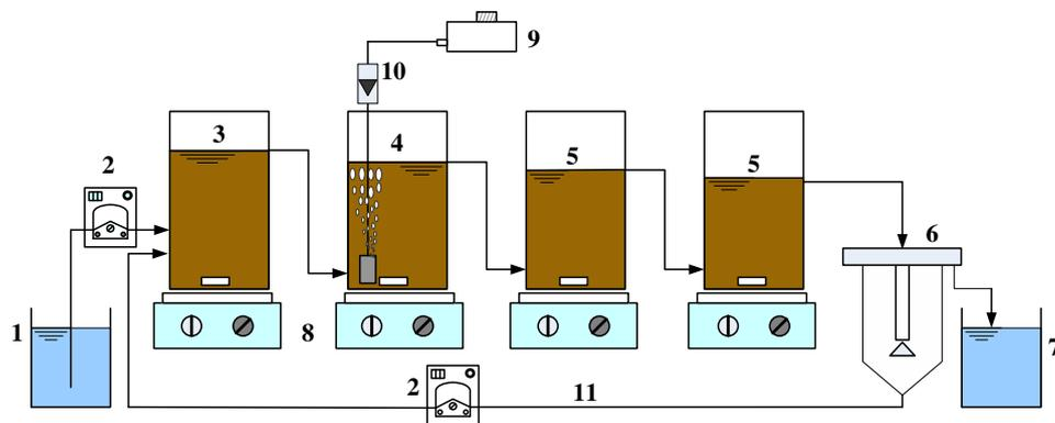
**Fig. 1.** Schematic diagram of the AOA process (Run 2). 1 – Influent tank, 2 – peristaltic pump, 3 – anaerobic basin, 4 – aerobic basin, 5 – anoxic basin, 6 – settler, 7 – effluent tank, 8 – mixer, 9 – air pump, 10 – air flow meter and 11 – return sludge.
