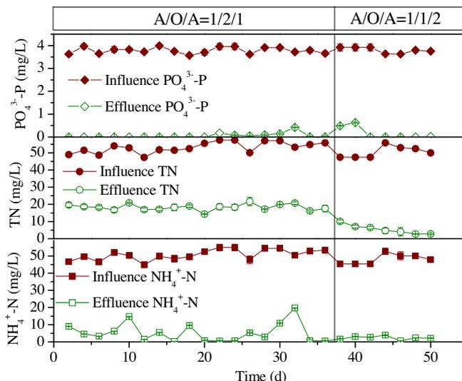
**Fig. 2.** Performance of the AOA process regarding  $\text{PO}_4^{3-}\text{-P}$ , TN and  $\text{NH}_4^+\text{-N}$  removal.
