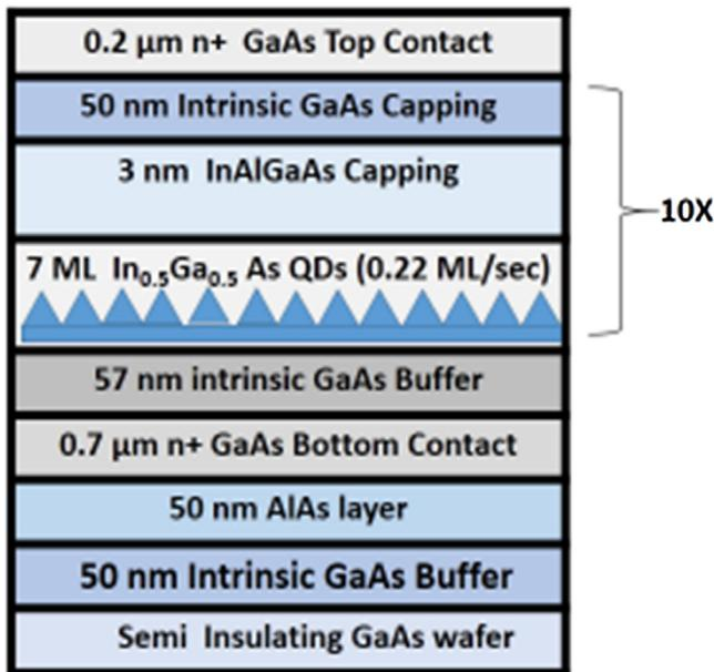
**Fig. 1.** Ten-layer quaternary alloy (InAlGaAs)-capped  $\text{In}_{0.5}\text{Ga}_{0.5}\text{As}/\text{GaAs}$  quantum dot infrared photodetector heterostructure.
