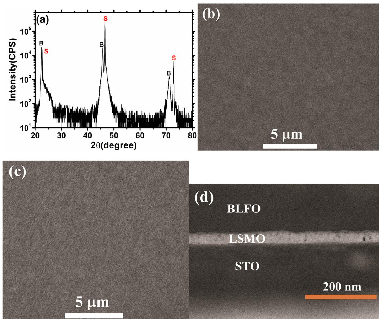
**Fig. 1.** (a) XRD patterns of BLFO thin films, S denotes STO substrate and B represents BLFO films. (b) SEM images of LSMO thin films. (c) SEM images of BLFO thin films. (d) The cross section scanning electron microscopy (SEM) image of BLFO/LSMO/STO sandwiched structure.
