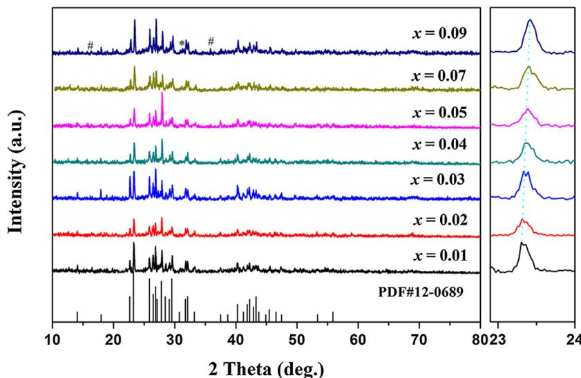
Fig. 1. XRD patterns of high- $\text{Ba}_{3-x}\text{P}_4\text{O}_{13}:\text{xEu}^{2+}$  ( $0.01 \leq x \leq 0.09$ ) samples.
