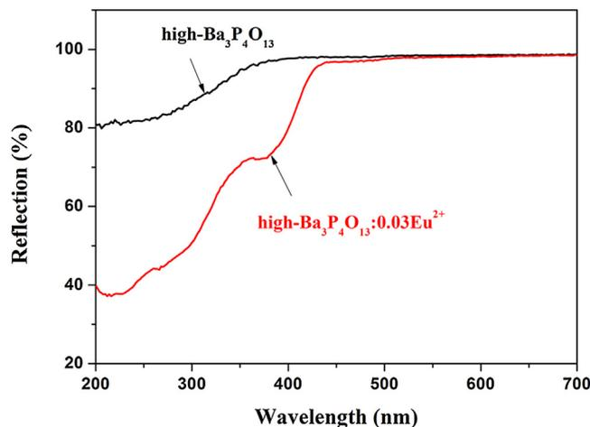
Fig. 2. DRS of doped and undoped high- $\text{Ba}_3\text{P}_4\text{O}_{13}$ .
