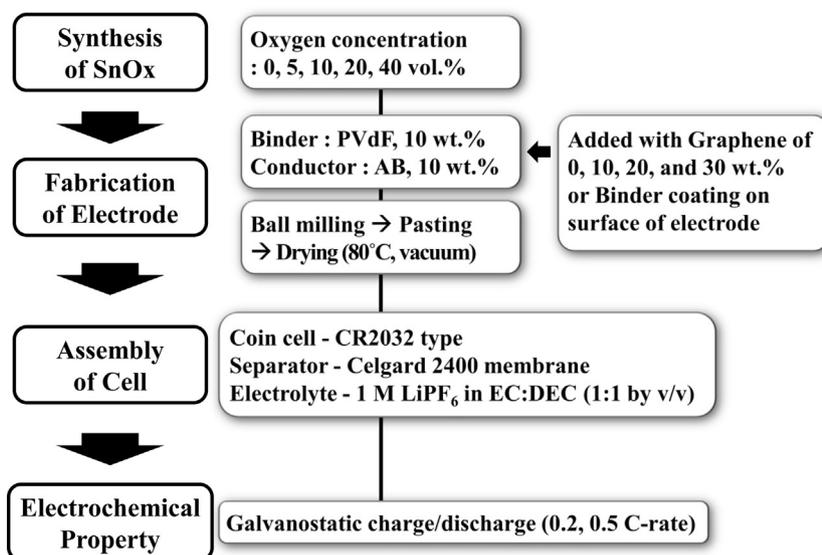
Fig. 1. Experimental flow chart of fabrication processes.
