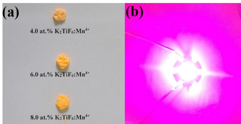
**Fig. 1.** (a) Photo of the obtained red-phosphors with various  $\text{Mn}^{4+}$  ions doping concentrations. (b) Red-emission image by using a blue-chip to excite the KTFM with a 3 V voltage.
