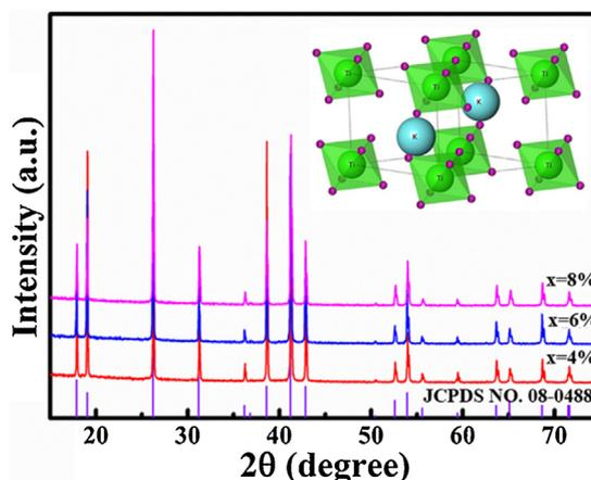
**Fig. 2.** XRD patterns of  $\text{K}_2\text{Ti}_{(1-x)}\text{Mn}_x\text{F}_6$  phosphors with different  $\text{Mn}^{4+}$  ions doping concentrations. The inset shows the crystal structure of  $\text{K}_2\text{TiF}_6$ .
