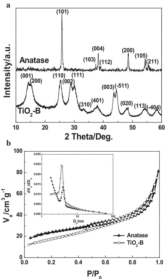
Fig. 1. (a) XRD patterns and (b)  $\text{N}_2$  adsorption–desorption isotherms (the inset pore size distribution curves) of Anatase and  $\text{TiO}_2\text{-B}$ .
