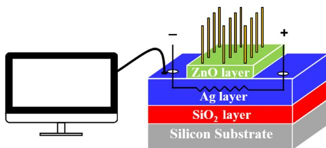
Fig. 1. Schematic illustration of EIC process on ZnO NRs/ZnO/Ag/SiO<sub>2</sub>/Si structure.
