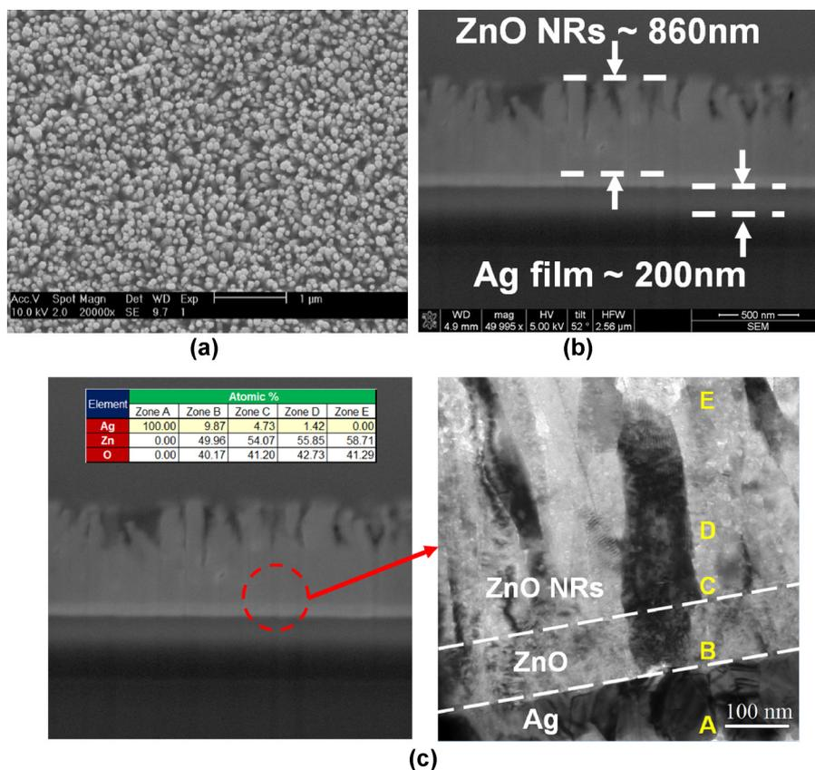
Fig. 2. Structural characterizations of the ZnO NRs/ZnO/Ag structure. (a) top-view SEM image; (b) cross-section and (c) TEM image of a ZnO nanorod arrays on ZnO/Ag layer.
