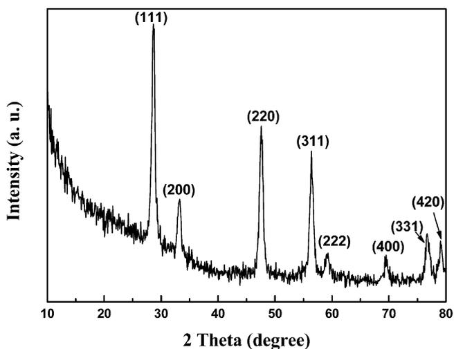
**Fig. 1.** XRD pattern of CeO<sub>2</sub> NPs prepared by the hydrothermal process at 180 °C for 100 min.
