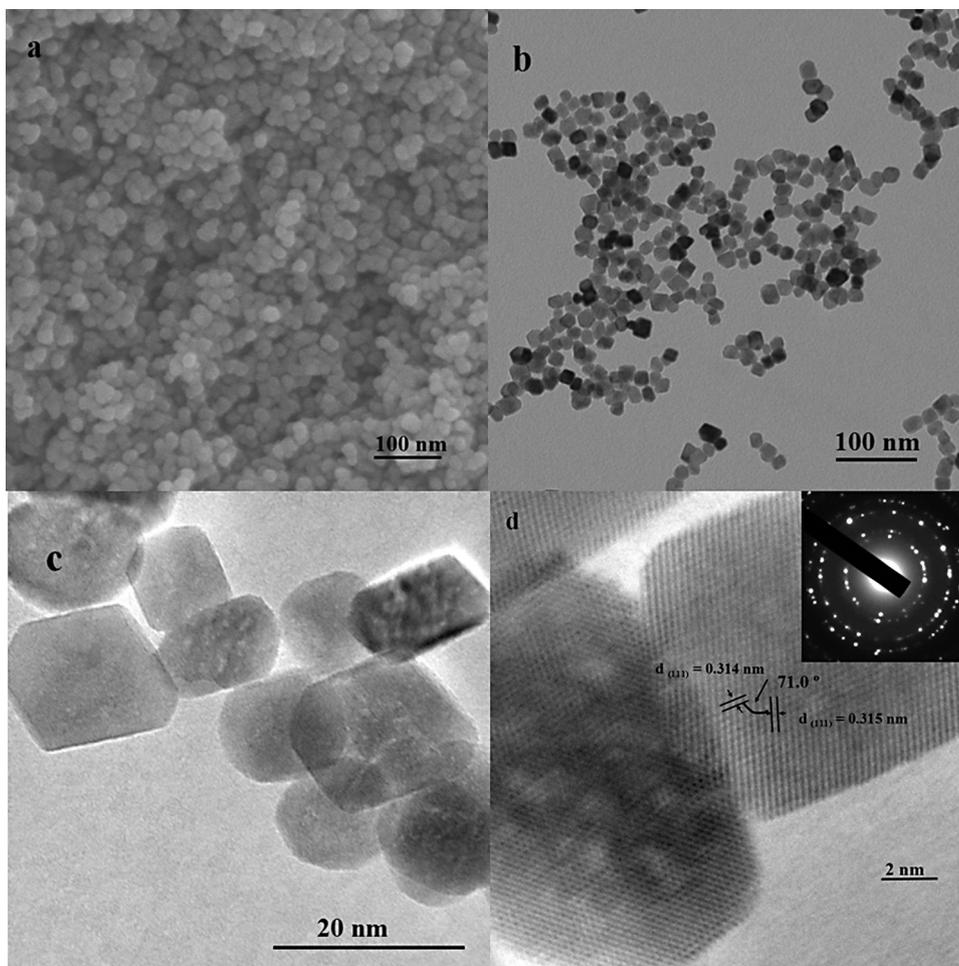
**Fig. 2.** (a) SEM image, (b, c) TEM images, and (d) HRTEM image of the typical CeO<sub>2</sub> NPs. The inset of (d) is the corresponding SAED.
