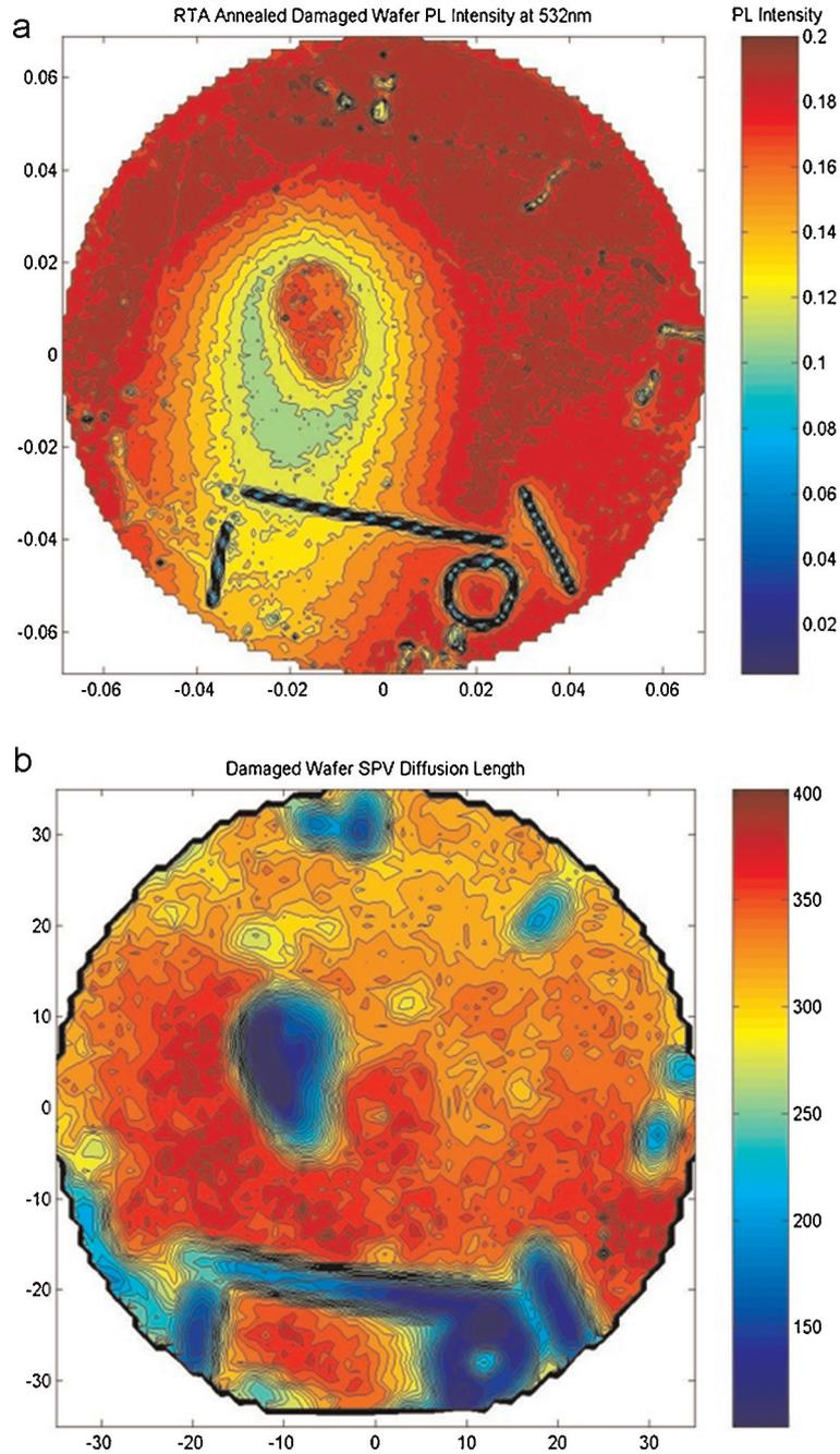
**Fig. 1.** (a) Photoluminescence and (b) SPV maps of a bulk Si wafer. Region A: touched with a finger, B: scratched with a metal pointer [10].
