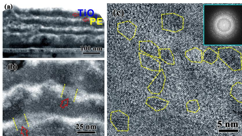
Fig. 2. TEM cross-sectional views of  $(\text{TiO}_2/\text{PE})_4$  nanolayered composite (a) at low magnification and (b) at high magnification. (c) HRTEM image of inorganic  $\text{TiO}_2$  layer, showing the existence of nanocrystallines.
