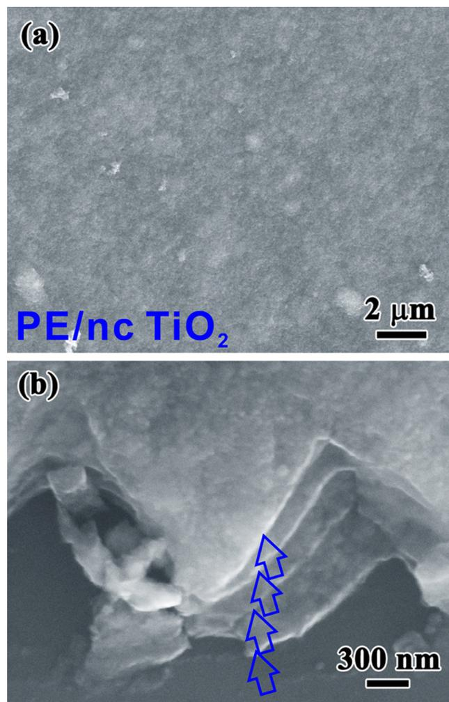
Fig. 1. SEM images of  $(\text{TiO}_2/\text{PE})_4$  nanolayered composite, (a) surface morphology and (b) layered structure.
