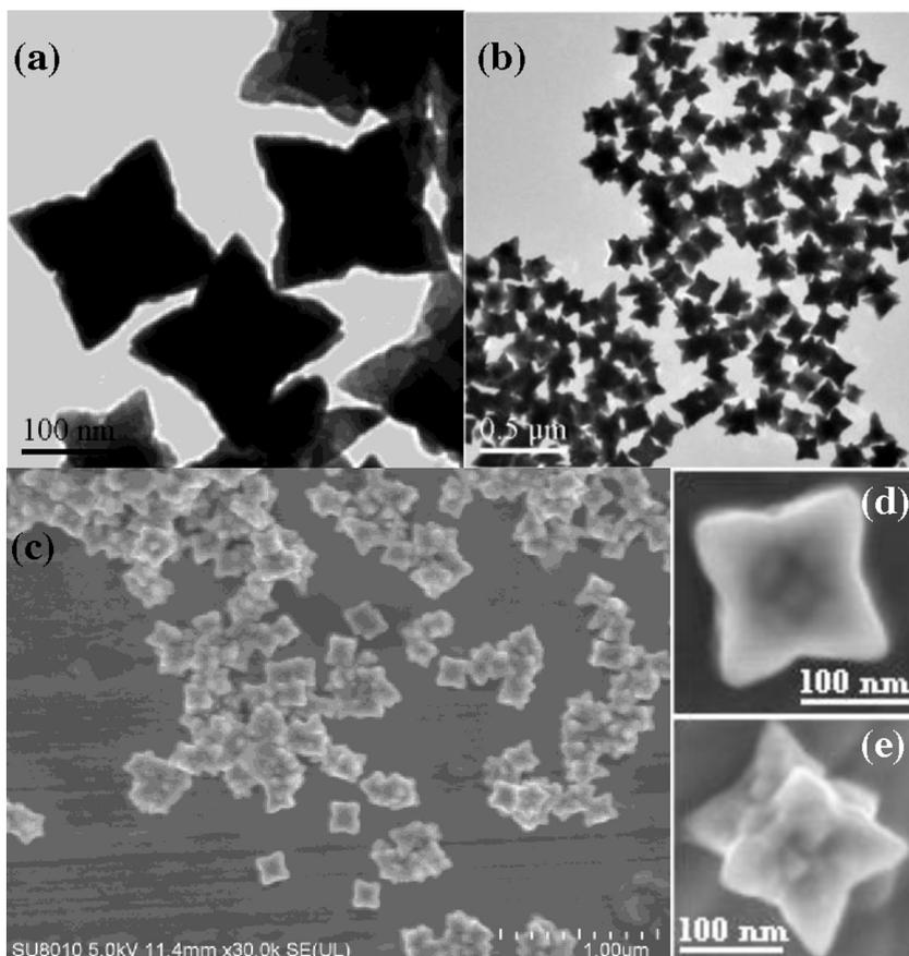
**Fig. 1.** TEM and SEM images of the as-prepared Pt octapods. (a and b) Typical TEM images; (c) typical SEM images; (d and e) SEM images of a single particle. [H<sub>2</sub>PtCl<sub>6</sub>] = 2 mmol L<sup>-1</sup>; H<sub>2</sub>PtCl<sub>6</sub>/KI/PVP was 1/30/45 (molar ratio).
