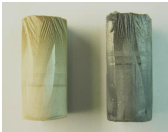
Fig. 1. Optical photos of porous GO (left) and RGO foams (right).
